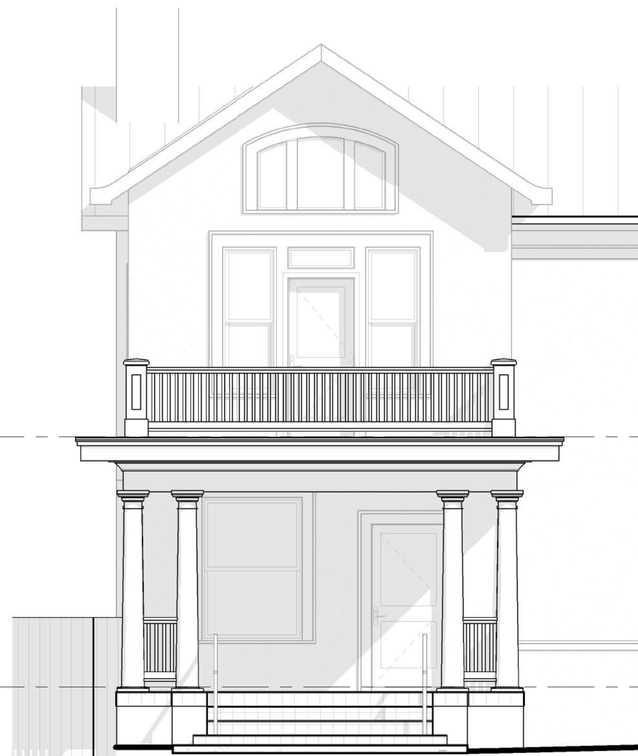
6 FRONT ENTRY - SOUTH ELEVATION (ARMY BLVD.) SCALE : 1/4" = 1'-0"
